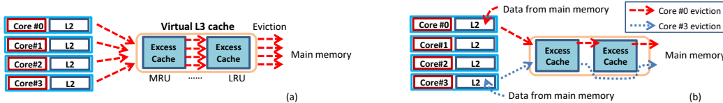
Figure 7. Static sharing scheme. (a) Homogeneous static sharing. (b) Heterogeneous static sharing.
