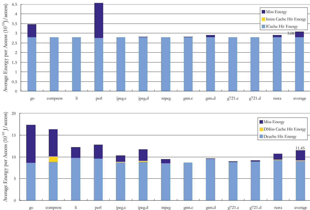
Figure 3. Breakdown of the average energy consumption per memory access. The upper graph is for instruction access, and the lower graph for data access. The energy for an on-chip cache miss is assumed to be 200.0 \times 10^{-10} J .
